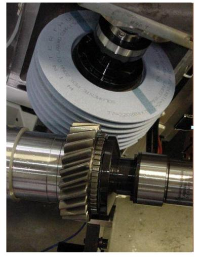
Fig. N°1 – Grinding with worm wheel
