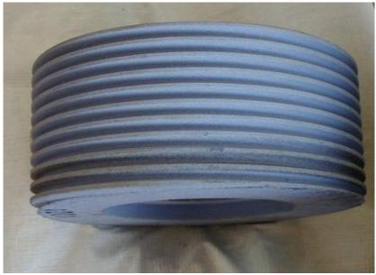
Fig. N°1- Grinding wheel in aluminum oxide
